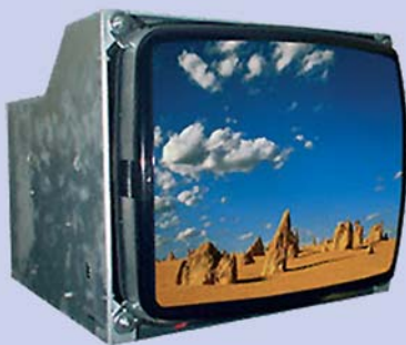
21" Vartech Open-frame CRT Displays Installed in Tarong Power Station Control Room.
